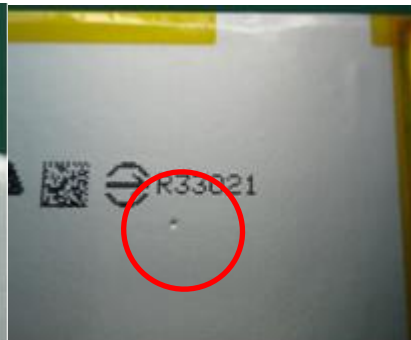
Dent on the Cell surface
